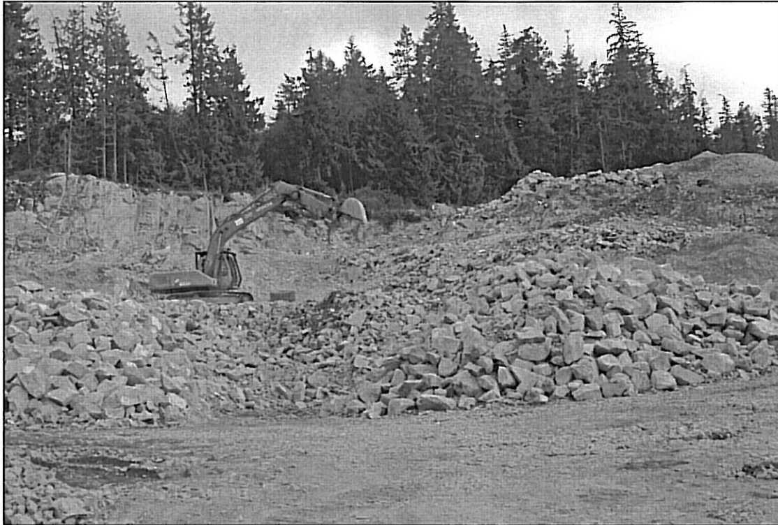
Picture 4: Quarrying Aggregate for Road Construction
